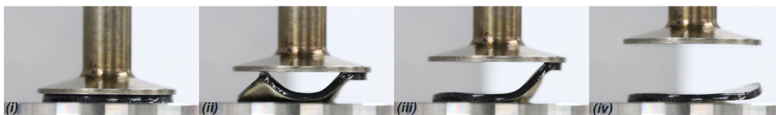
Fig. 4. Photos showing the process of GSDZ hydrogels stretching and detaching during rheo-tack measurements.
