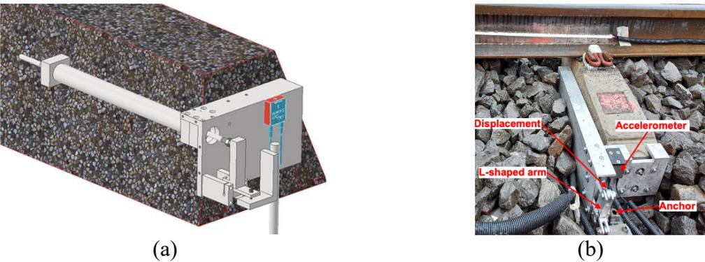
Figure 25. Detail of sleeper containing a vertical base plate, an L-shaped mechanism, one accelerometer and one displacement transducer. (a) The designed setup, (b) overview of an instrumented sleeper with an accelerometer and a displacement transducer. The positions of the anchor tip and the L-shaped mechanism with a swivel and a roller are shown
