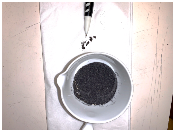
Fig. 6. Partial agglomeration of the braunite oxygen carrier.
