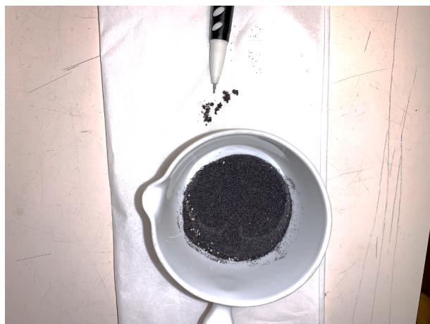
Fig. 6. Partial agglomeration of the braunite oxygen carrier.
