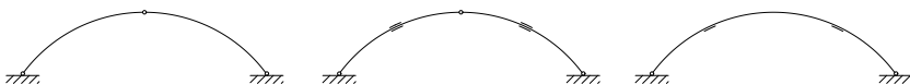
Figure 2.6: Structural systems for arches: three hinged arch, three hinged arch with interior joints, two-hinged arch and interior joints
