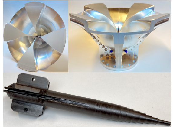
Fig. 1: QRFH and the polyimide load insert (magnified).
