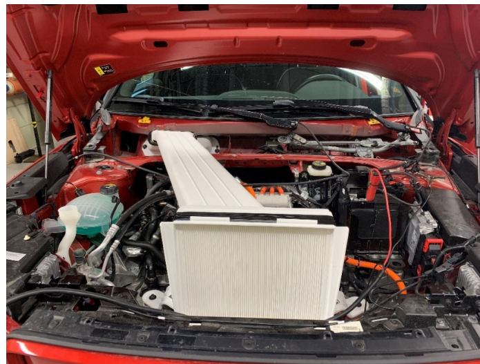
Figure 6 Filter prototype installation in an existing production vehicle's thermal bay
