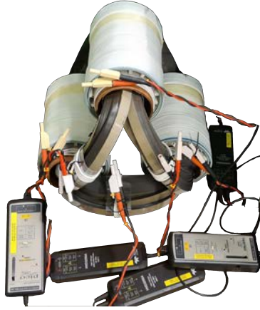
Figure 8.7: The experimental setup for measuring flux waveforms.
