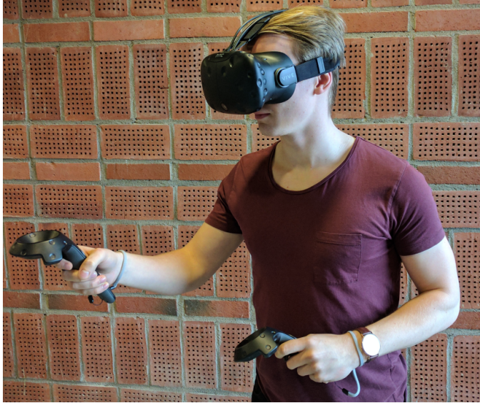
(a) A figure showing a person wearing a VR-headset consisting of an HMD and two hand-held controllers.
