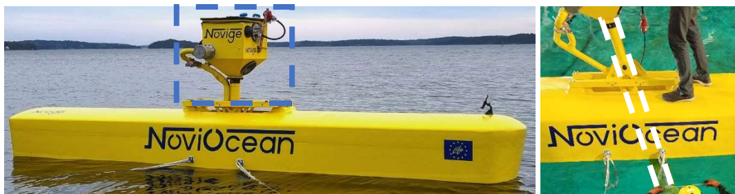
Figure 5. Components of NoviOcean WEC (Novige, 2023a): the water turbine in the blue dashed box and the hydraulic cylinder in the white dash box.
