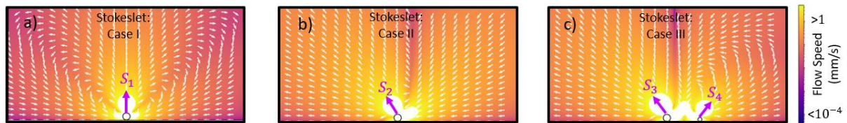
Figure 8: Stokeslet simulations of Marangoni flow induced by a) Case I: a single bubble with a temperature gradient normal to the interface and b) Case II: a single bubble with temperature gradients both perpendicular and parallel to the surface c) Case III: by two unequal nearby bubbles with an additional temperature gradient parallel to the surface.
