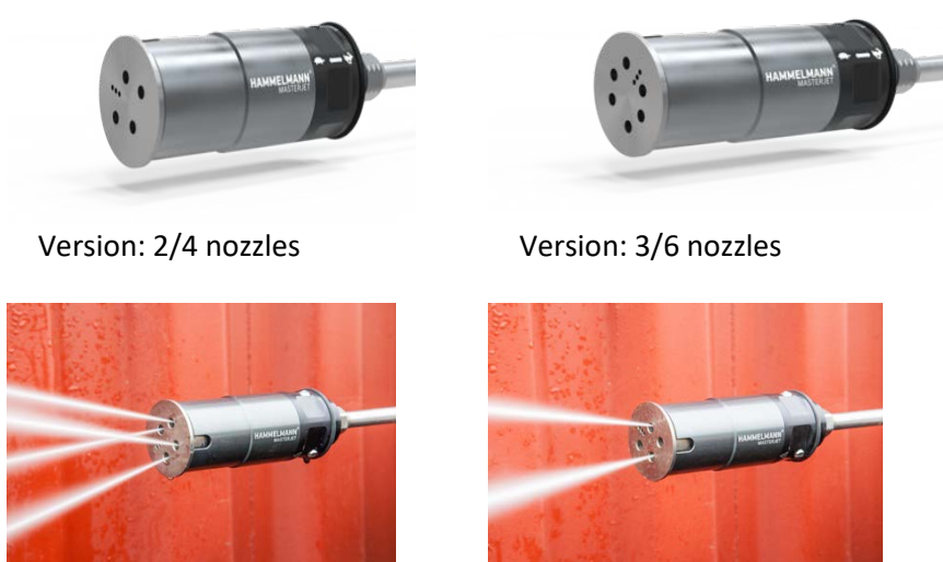
Figure 13. Example of water jet tips for underwater hull cleaning. Different nozzle configurations operate under pressure 1800-3200 bar and flowrate up to 60 LPM (Hammelmann)
