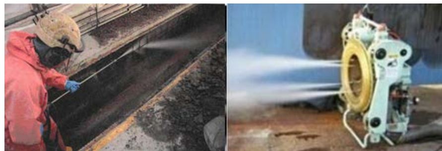
Figure 15. Non cavitation water jet system (left)[2], High-pressure water cleaning jet technology (right) ( HullWiper )
