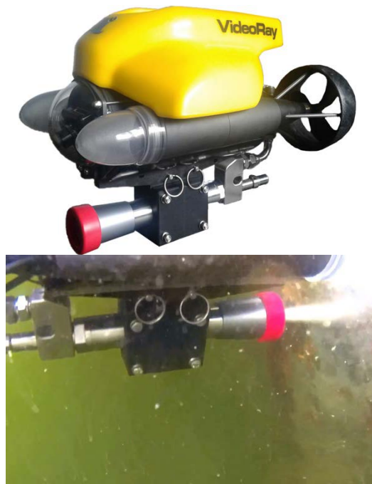
Figure 14. Waterjet cavitation cleaning with ROV ( DiveWise )
