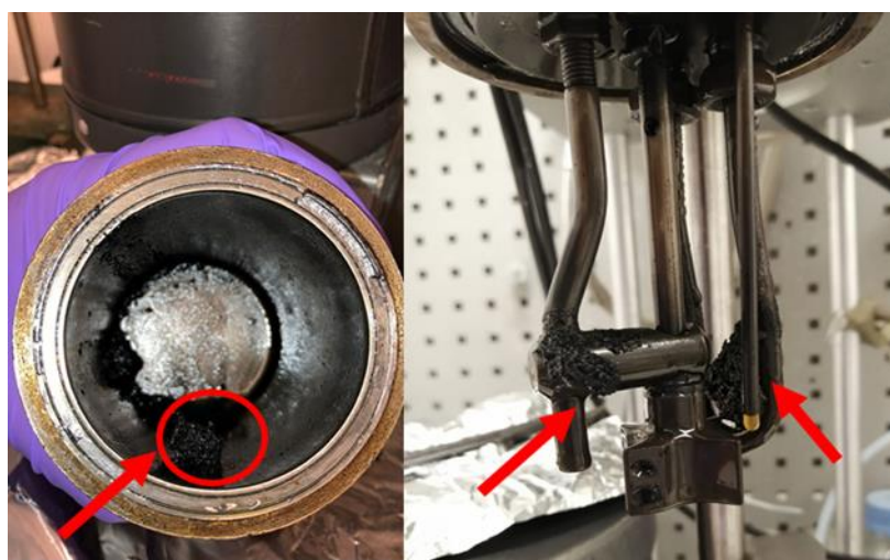
Figure 40. Solid residues resulting from non-catalytic experiments of co-hydrotreatment of KL. Left: inside of the reactor vessel. Right: reactor head with a stirrer, thermocouple, dip tube, and cooling coil.
