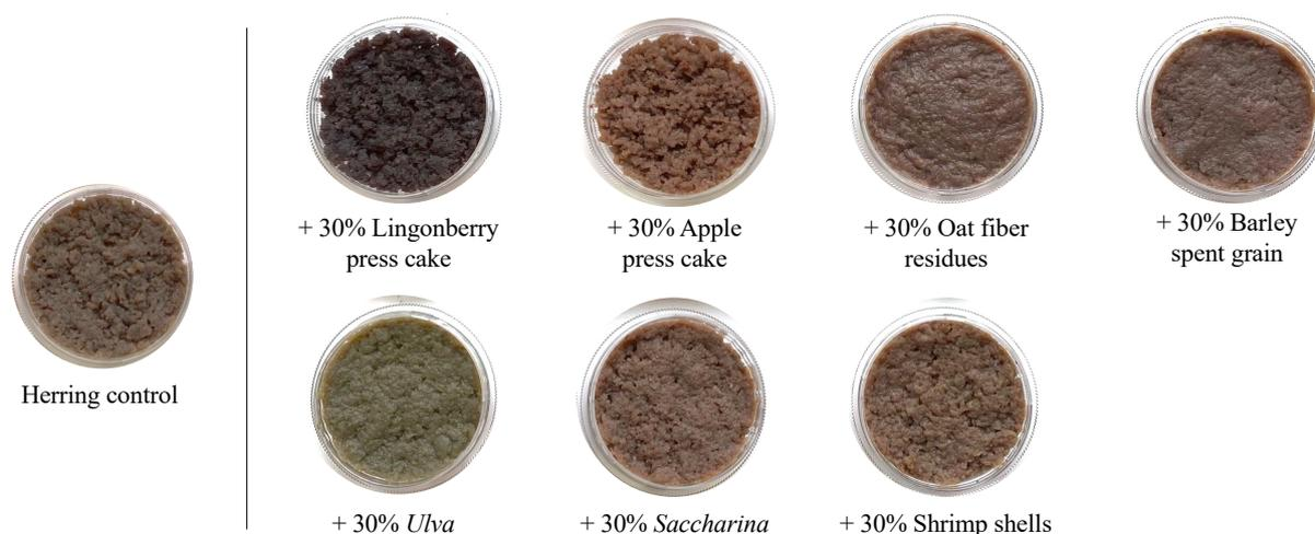
**Figure 5.3:** Color of protein isolates produced from herring co-products in the absence and presence of helpers by the alkaline version of pH-shift process. The protein isolates have a pH of 7 and a moisture content of 80%.
