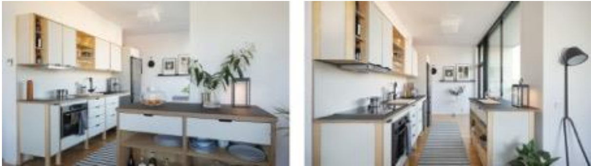
Figure S.5. Prototype kitchen installed in living lab, featuring a modular plywood construction and moveable kitchen island to adapt to changing social settings and functional demands.
