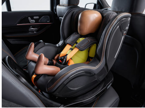
Fig. 9 Networked child seat with PRE-SAFE® functions
