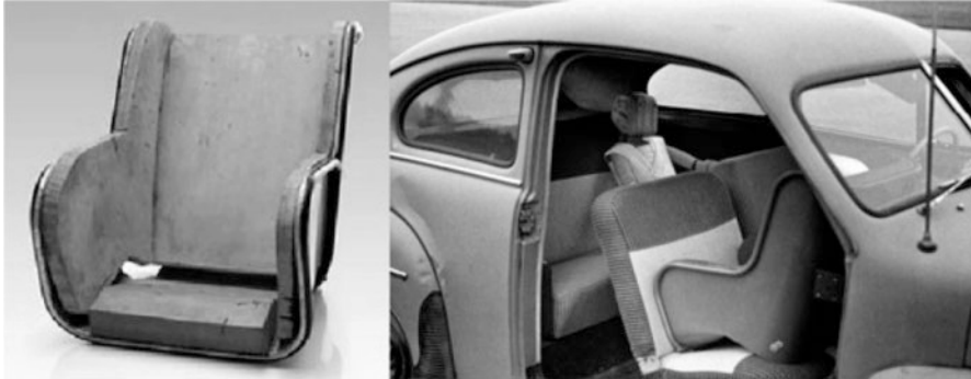
Fig. 9 Early rearward-facing child restraint prototype
