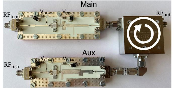
Fig. 14. Photograph of the fabricated CLMA prototype circuit.
