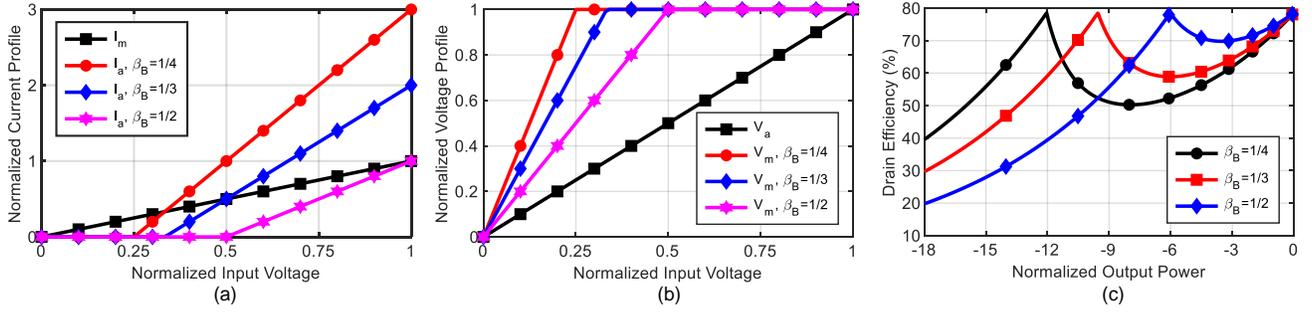
Fig. 4. (a) Normalized amplitude of the fundamental currents and (b) normalized amplitude of the fundamental voltage from the Doherty PA versus normalized input drive voltage, for  $\beta_B = 1/4, 1/3,$  and  $1/2$ . (c) Drain efficiency of the Doherty PA, versus normalized output power, for  $\beta_B = 1/4, 1/3,$  and  $1/2$ .
