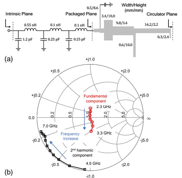
Fig. 10. (a) Continuous-mode output matching network with the equivalent parasitic and packaged model of the CGH40010F transistor. (b) Simulated matching results of the output network with a reference impedance of  $R_{opt}/\beta$ .
