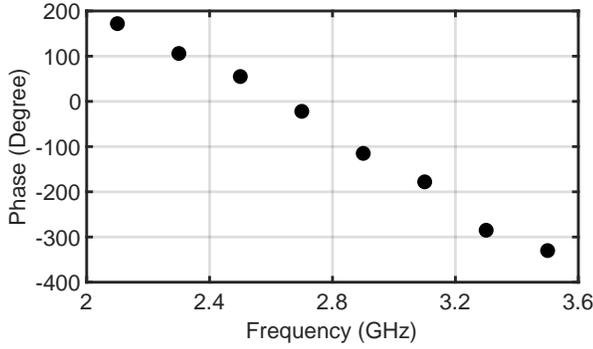
Fig. 15. Optimal phase shift between the main and auxiliary branches across designed frequencies for maximized back-off efficiency.
