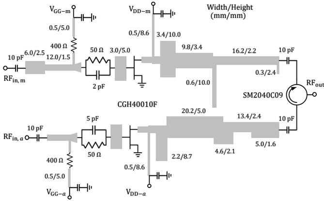
Fig. 8. Circuit schematic of the proposed circulator load modulated amplifier.
