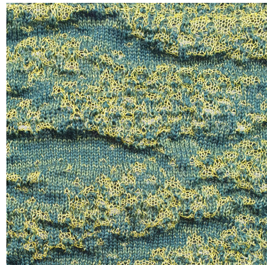
Figure 2-14 False lace pattern. Left: an illustration of the principle of the knit. Right: a section of a prototype knitted with the technique, using wool (dark green) and linen (yellow) yarns
