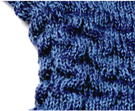
Figure 2-12. Tuck stitch knit. On the left is an illustration of the principle of a tuck stitch and on the right is a prototype knitted with wool yarns.
