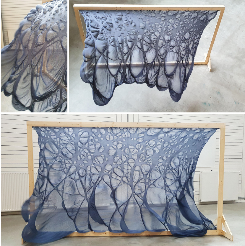
Figure 4-2. The large-scale drop-stitch prototype with wind applied, shown with two different mountings.
