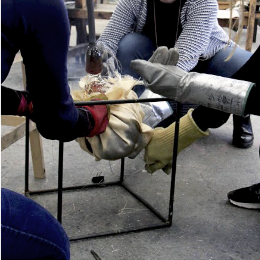
Figure 3-4. Glass blown into a textile mould mounted on a steel frame.
