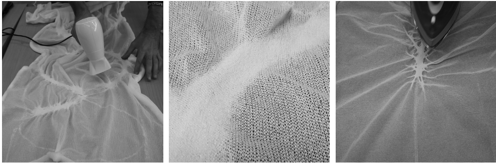
Figure 2-11. Single jersey heat changing textiles. Left and middle: Trevira CS PEMOTE®, modified with hairdryer. Right: COMFIL® PET modified through ironing.
