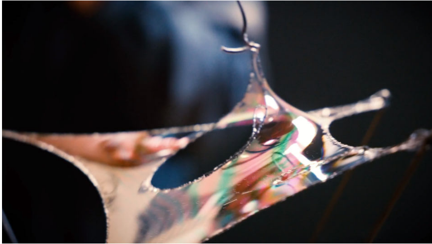
Figure 2-2 A soapfilm model as a conceptual model for a tensile structure.
