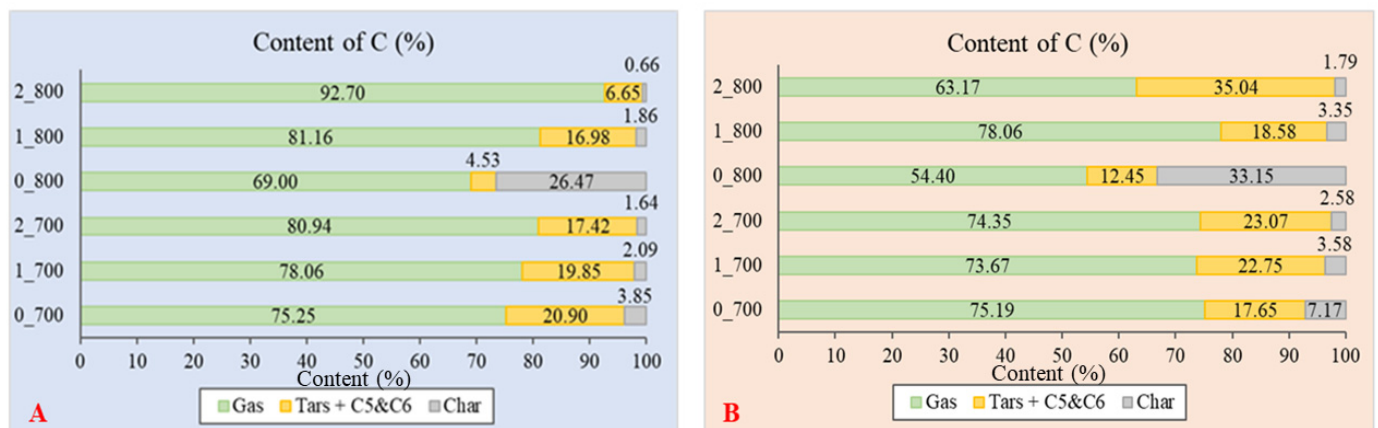
Figure 7. Carbon (%) distribution in the gas, tars, and char phases originated from the 3PFM (A) and KN95 (B) face mask steam gasification (y-axis corresponds to the SCR_temperature of the process).
