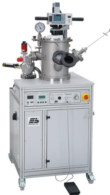
Figure 4.1. Arc melter from Edmund Bühler GmbH.
