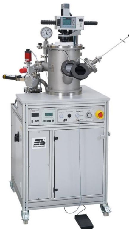
Figure 4.1. Arc melter from Edmund Bühler GmbH.
