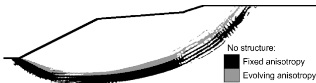
Figure 7. Failure surfaces, here represented as total deviatoric strains, from simulations without destructuration.
