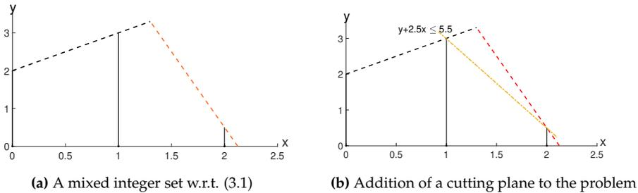
Figure 3.1: Mixed integer set and a cutting plane
