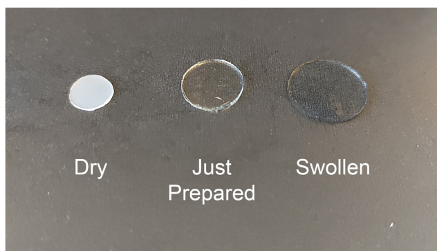
Figure 12. Appearance of the hydrogel discs used throughout the work. The dry hydrogel (left) is after 5 days of drying at 40 °C, where only the polymer remains. The just prepared hydrogel (middle) is the appearance just after it has been punched out from a sheet. The swollen hydrogel (right) is the appearance after being stored in excess water for 3 days, which is the most used version.
