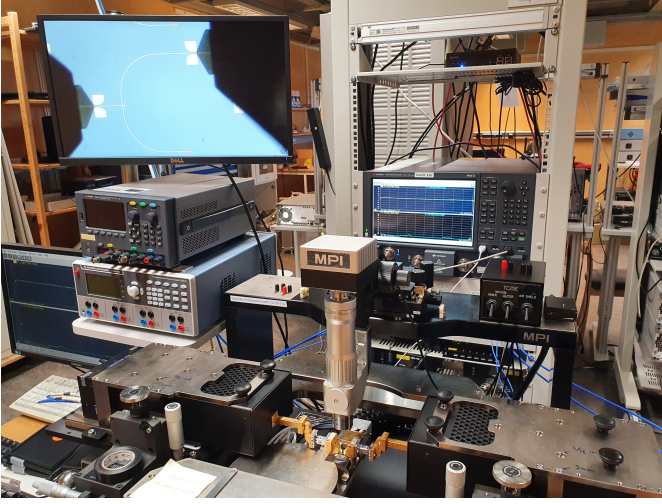
Fig. 6. Photograph of the measurement setup based on a probe station, a vector network analyzer, frequency extenders and T-Wave ground-signal-ground probes.
