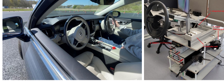
Fig. 1. Left: Test vehicle with the two steering systems. Right: Desktop test rig with the feedback motor and the steering rack
