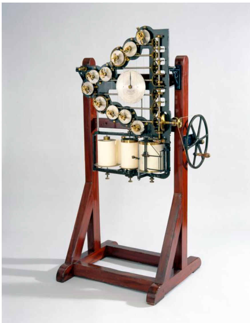
Figure 1.5: Thompson's tide predicting machine at the Science Museum, South Kensington, London [36]
