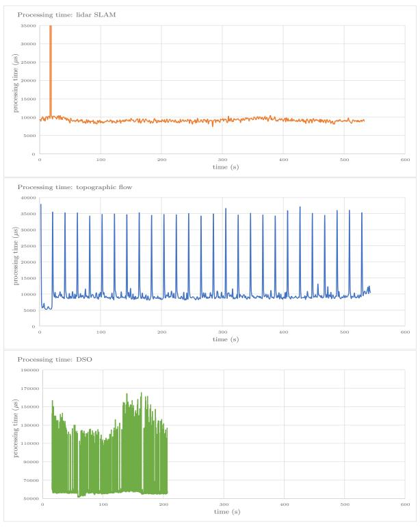
Figure 5.7: The performance time of each processed result for the lidar SLAM, topographic flow, and DSO algorithms. At  $19\,\mathrm{s}$ , there is a spike in processing time of the lidar SLAM which reached  $1.2\,\mathrm{s}$ . As with the angular rotation shown in Fig. 5.6, the DSO results stop after  $210\,\mathrm{s}$ .
