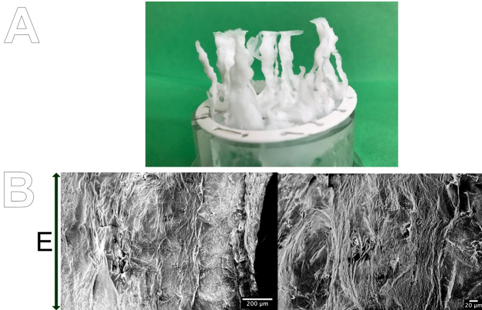
Figure 5.17 (A) Structures obtained from the electro-osmotic dewatering of TEMPO-MFC at 24 V/cm; SEM micrographs at different magnifications. (B) Scale bars, from left to right: 200 and 20 \mu\text{m} .
