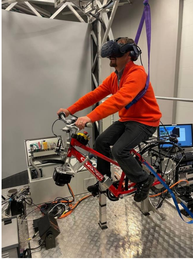
Figure 4- Bike simulator with virtual reality headset
