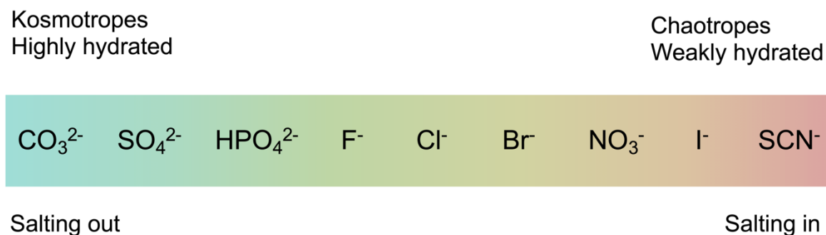
Figure 4 Hofmeister series of anions, from left to right the hydration of ions decreases.
