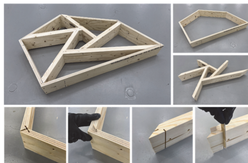
Figure 2 Top: Timber system including the polygonal frame and reciprocal beams. Bottom: using wooden splines for aligning elements in a configuration
