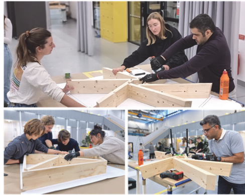
Figure 13 Easy and rapid alignment and assembly of the polygonal and reciprocal beams
