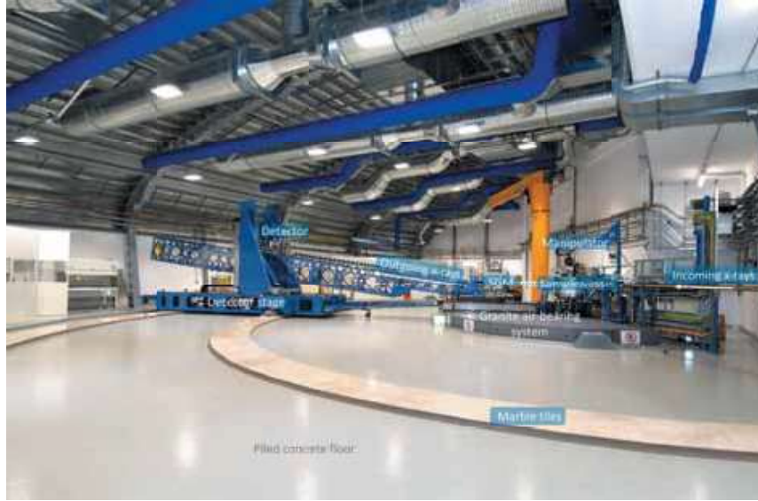
Figure 2.5: Spectrometer image. RIXS spectrometer at the I21 beamline of the Diamond Light Source. From Ref. [25].
