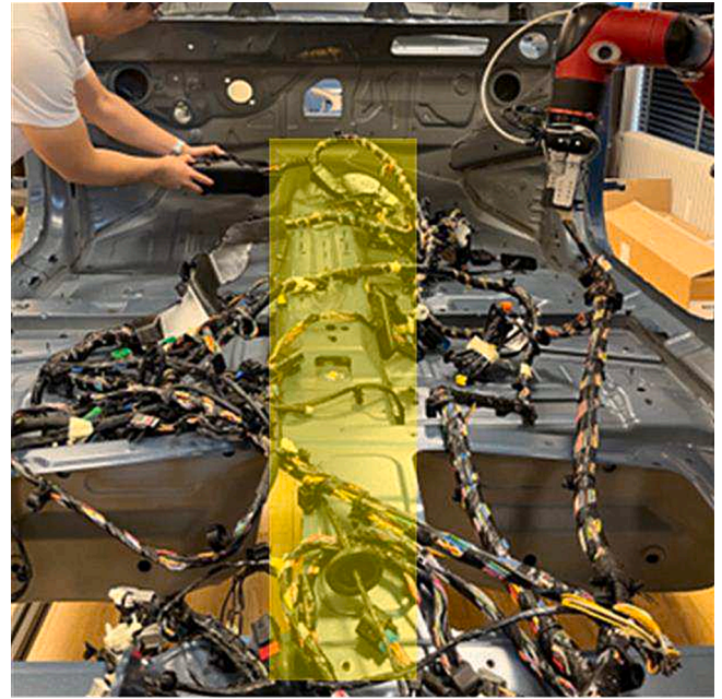
Fig. 9. Operator and a Robot Collaborating in a Wire Harness Assembly Process with Y-Axis Highlighted.
