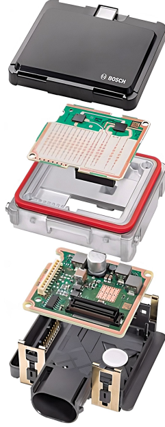
Figure 2.4: Exploded view of the Bosch RADAR sensor [51].
