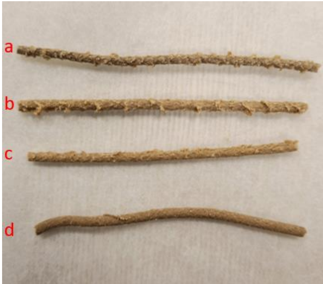
Figure 11. A visual impression of filaments composed of a) PP-TMP b) PP-TMP AKD Hex c) PP-TMP AKD Lau and d) PP-TMP AKD St, as compounded for 10 minutes and extruded at 150 kN and 190 °C.
