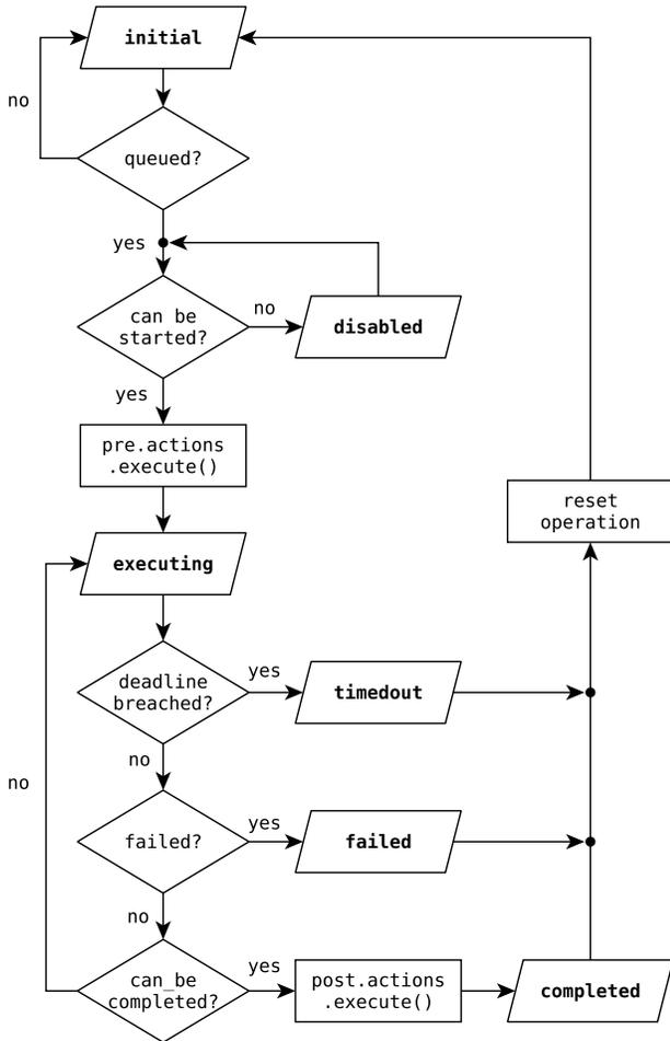
Fig. 4. An operation and its states while being executed by the runner.
