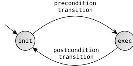
Fig. 1. A model of an operation.
