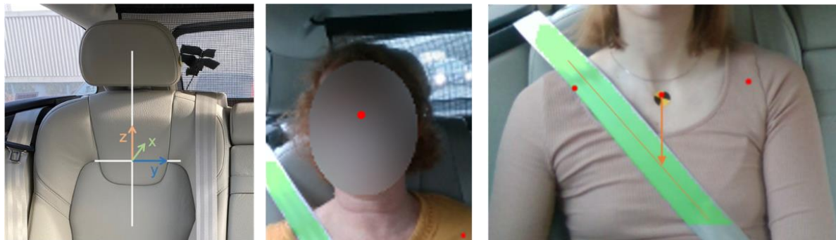
Figure 2. Definition of the coordinate system (left), head position (centre), and upper sternum position (right) as well as shoulder belt distance (right).
