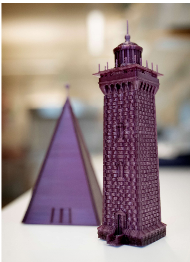
Figure 5.2. Photo of 16 and 20 cm tall miniature versions of the Vinga beacon and lighthouse 3D-printed with PMMA:Au nanosphere filament. Photography by Malin Arnesson/Chalmers.
