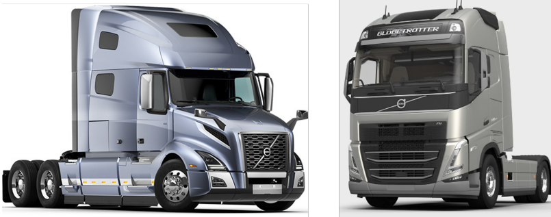
Figure 4.3: Variation in cab geometry in Volvo Truck products offered in North America (left) and Europe (right)
