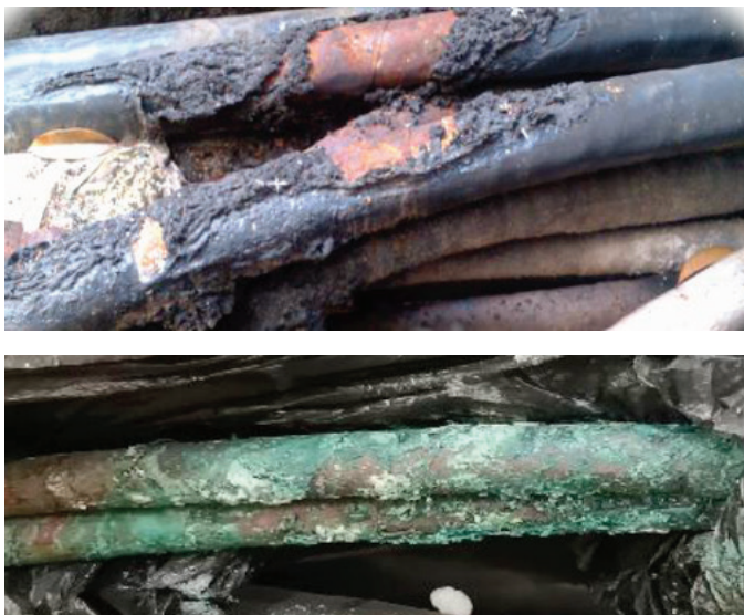
Figure 13 common damages found at cable body, top: third party damages; bottom: water damages.
