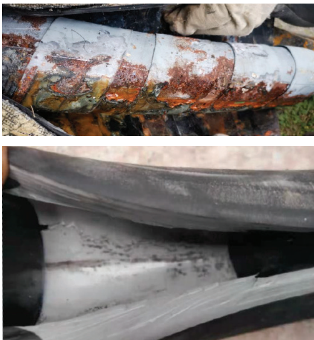
Figure 11 Examples of failure damages appeared at MV cable accessory interfaces due to multi-physical stresses combined with water ingress.
