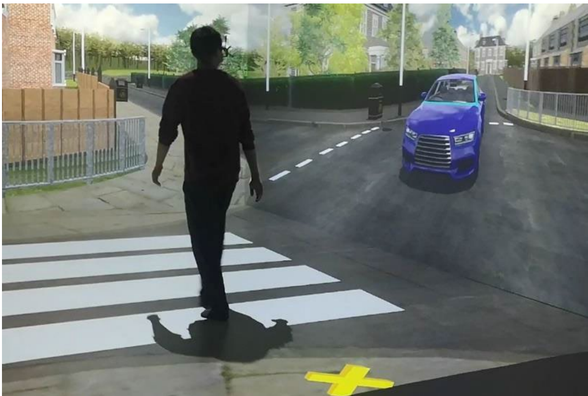
Figure 6. Interaction between the pedestrian and the AV with the eHMI on, at a zebra crossing, in the pedestrian simulator lab. The yellow cross indicates the pedestrian's starting position at the curb (adapted from Yang et al., 2023).
