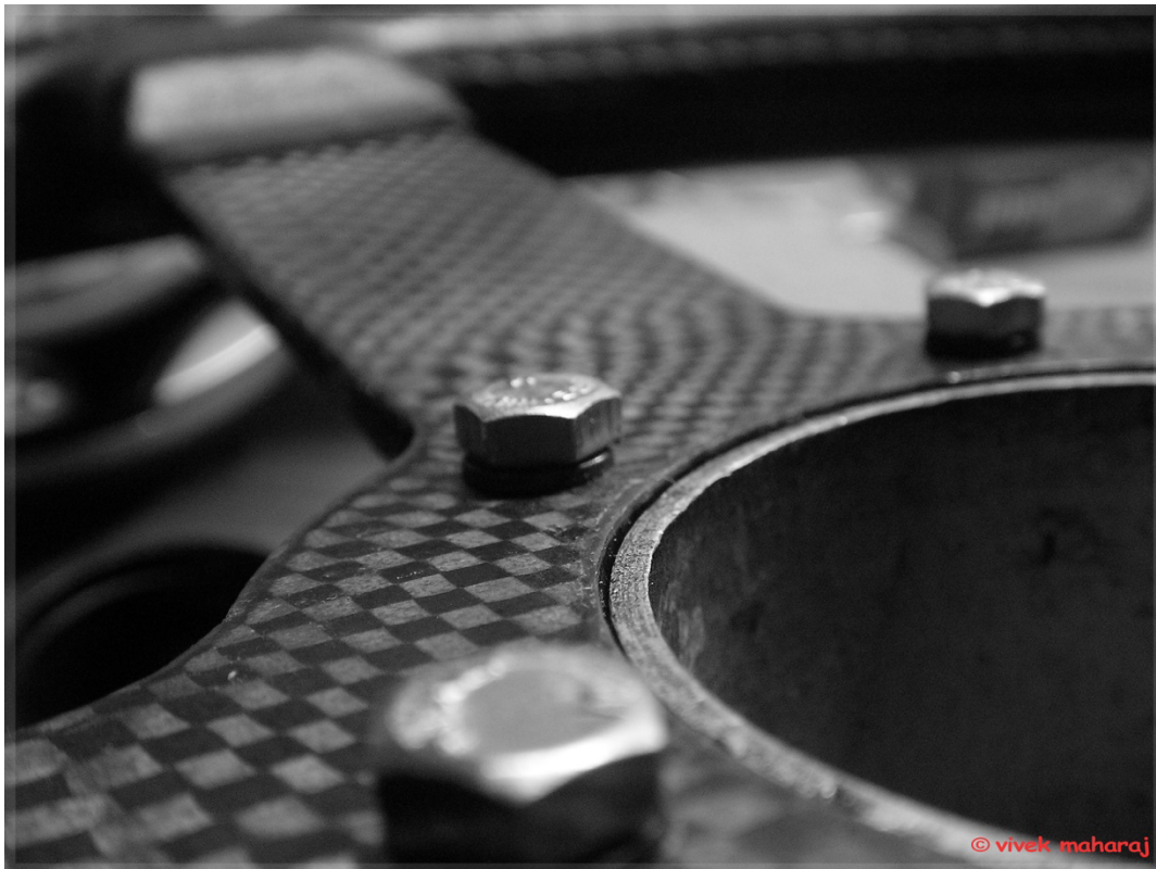
Figure 2. A steering wheel made from carbon fibre composites. The checked pattern illustrates the woven fibre, which is impregnated with a polymer. Reprinted under licence CC BY 2.0 1 .
