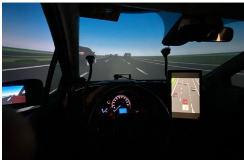
Figure 2 Interior of DAVSi driving simulator with designed user interfaces
