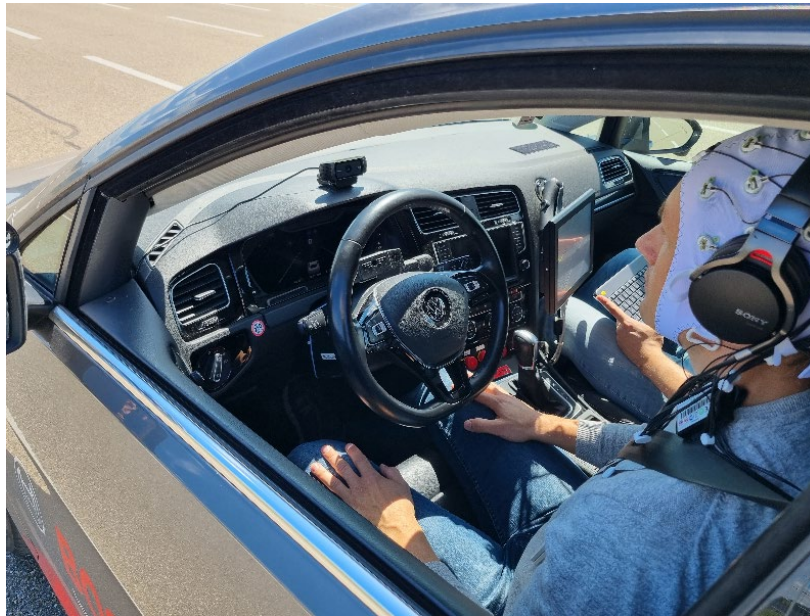
Figure 2 Using EEG to record brain responses to novel environmental auditory cues in a prototype of an automated vehicle on a test track in Renningen, Germany
