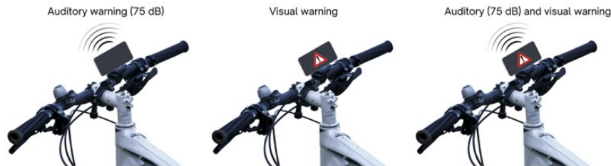
Figure 2. The auditory, visual, and visual-auditory warning system features of CycleSafe
