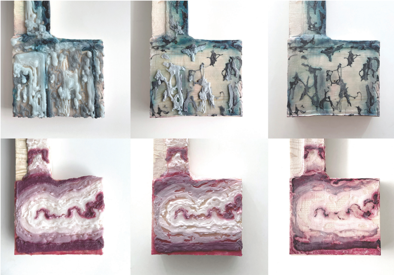
12 Aesthetic and geometric transitions of the new material layers from microfibrillated cellulose hydrogel seen in detail over time for the two different toolpath variants (from left to right: 3, 18 and 36 hours post 3D printing).
