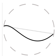
Figure 2.1: Illustration of how the length (dotted line) of a fiber (black) is defined.
