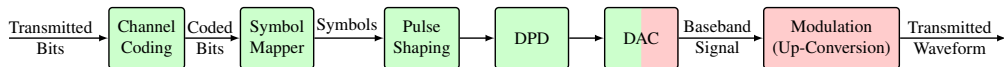
Figure 2.2: Block diagram of a conventional transmitter. Blocks highlighted in green operate in the digital domain, while the rest (i.e., blocks in red) operate in the analog domain.
