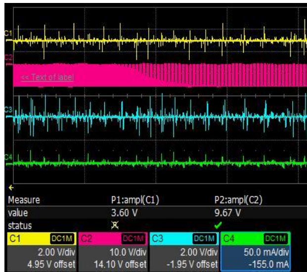
b) Test result of case B2 (bearing ground and main shaft floating).
