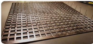
Figure 4.1: Needle panel used to generate charges in air.
