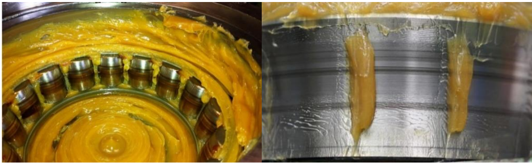
Figure 1.11: Wind turbine main shaft bearing lab test in SKF.
