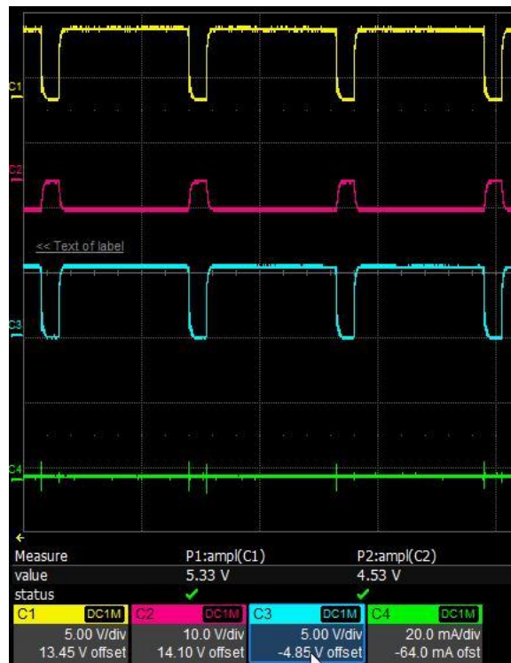
b) Test result of case B4 (both bearing and main shaft floating).
