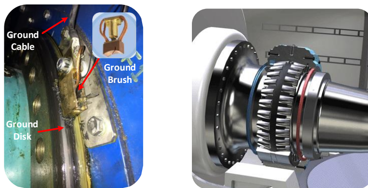
Figure 3.4: Typical ground brush and wind turbine main bearing.
