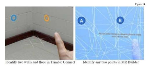
Examples of two- and three-point alignment in commercial BIM-AR viewers.
