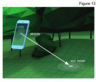
Hit-testing in WebXR will return the underlying plane (surface).
