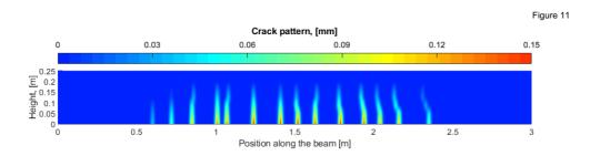
Comparison of crack width computed by DOFS strains and measured by DIC.
