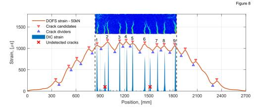
Determination of crack location based on DOFS and comparison with crack pattern from DIC.
