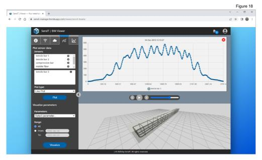
Inspection of raw sensor data in the project inspection page of the SensIT Manager web app for the cast study beam.
