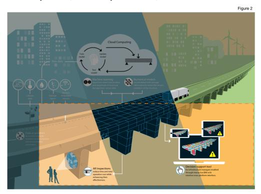
Infographic illustrating the different elements of the project "Sensor-driven cloud-based strategy for infrastructure management (SensIT)" and how they are linked to each other. The area highlighted in orange indicates the focus of the current project.
