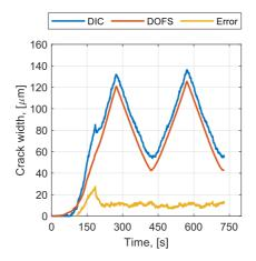
Comparison of crack width computed by DOFS strains and measured by DIC.
