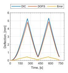
Comparison of beam deflections computed by DOFS strains and measured by DIC.
