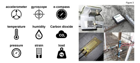
Different types of properties that can be measured by commercially available sensors (left). Example of different types of sensor for concrete structure applications, from top
