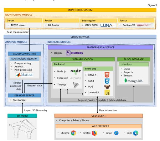
Schematic representation of the web-based asset management system's architecture.
