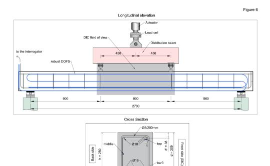
Geometry, loading setup and DOFS installation configuration for the RC beam specimen.
